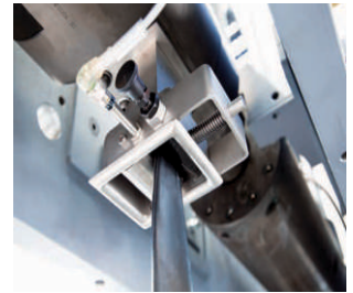
ActiveFeed - Actively driven feed roller
