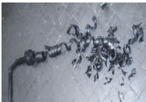
Vulcanized material pulled out of the PlastControl injection unit (nozzle, injection and screw cylinder)
