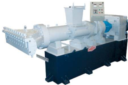
Rubber Strainer with Feeder Roller ▼ Range: 4" to 10" with Optional Dual Head
